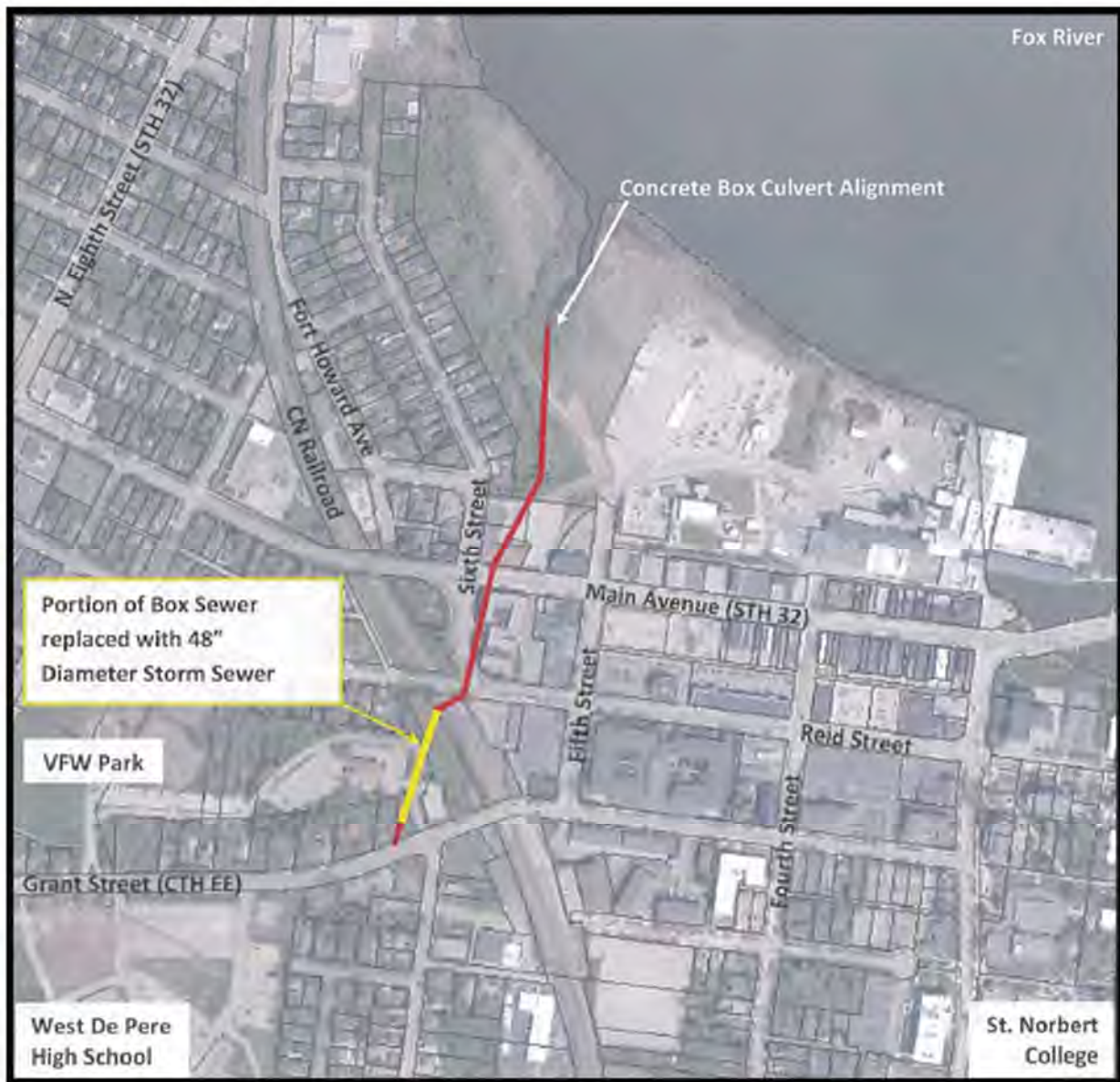
Figure 2 – De Pere Box Culvert Repairs
